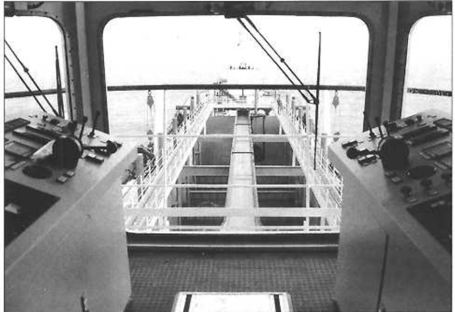
The dredgemaster's console provides an unobstructed view to the hopper section
