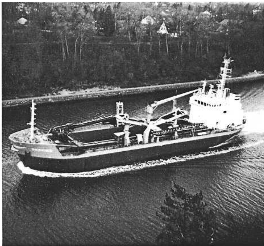
Trailing-suction hopper dredger mv Seekies , built at the Rendsburg yard of HDW Nobiskrug and fitted out by Krupp Fördertechnik at Lübeck
